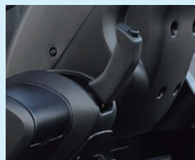
Parking brake lever (double action type)
