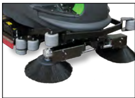
PRE-SWEEP SYSTEM ON CYLINDRICAL MODEL
