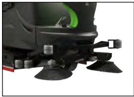
PRE-SWEEP SYSTEM ON CYLINDRICAL MODEL
