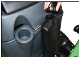
SEPARATE DETERGENT DOSING SYSTEM
