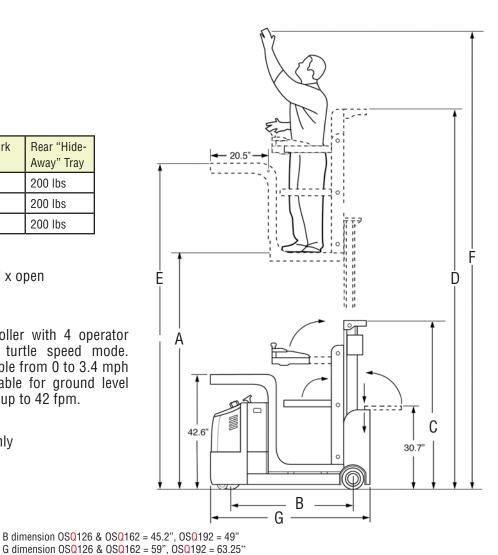
Lift Col Extended Load Tray Working Model # Mast Height Height Height Height Height F С D Ε A OSQ126 Triple Stage 64.9 159.0 203 126 180.9 Triple Stage OSQ162 83.9 239 162 237.9 195.0
