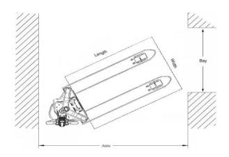
Aisle dimensions listed above assume 4" between loads. Use the larger dimension; load width or load length. For ease of use and add 6" to 12" for operator clearance to the appropriate specifications listed above. Truck performance may vary due to application requirements' and changes in model design.
