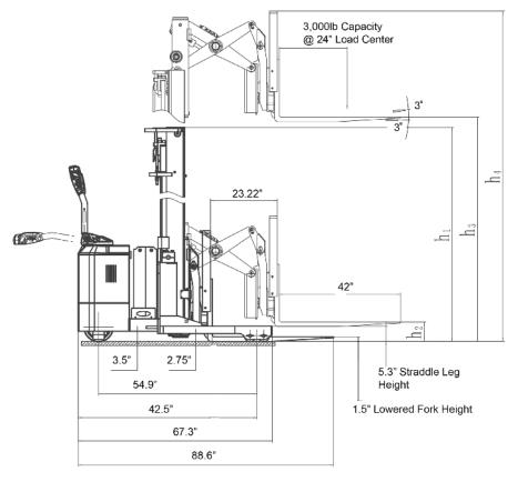
Overall length increased by up to 3" when control handle is perpendicular to the direction of travel
