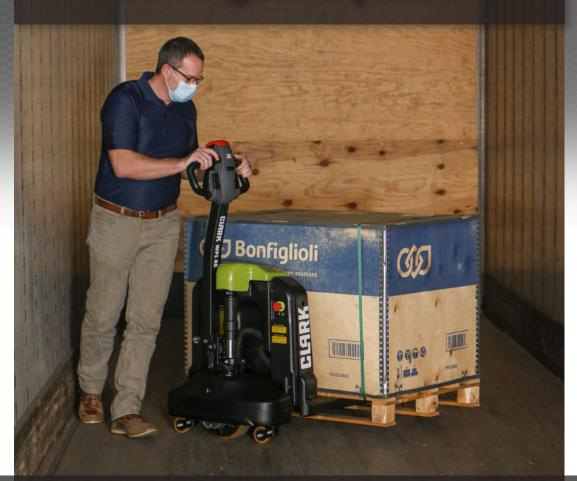
The WPL40 gives operators an electric pallet jack designed to work in closequarters with heavy loads. With the handle in the fully upright position, the WPL40 pin wheels in and out of tight spaces using a smaller, tighter turn-radius. With a 4,000 lb lift capacity, it moves and lifts loads with ease.
