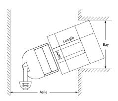
Aisle dimension listed above assume 4" between loads. Use the larger dimension; load width or load length. For ease of use and add 6" to 12" for operator clearance to the appropriate specifications listed above. Truck performance may vary due to application requirements and changes in model design.
